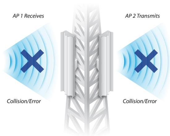
With GPS Sync, the APs transmit at the same time and receive at the same time, eliminating co-location interference.
