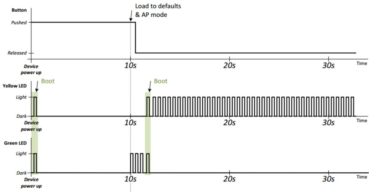
Figure 32 - LED indication when restoring factory defaults
