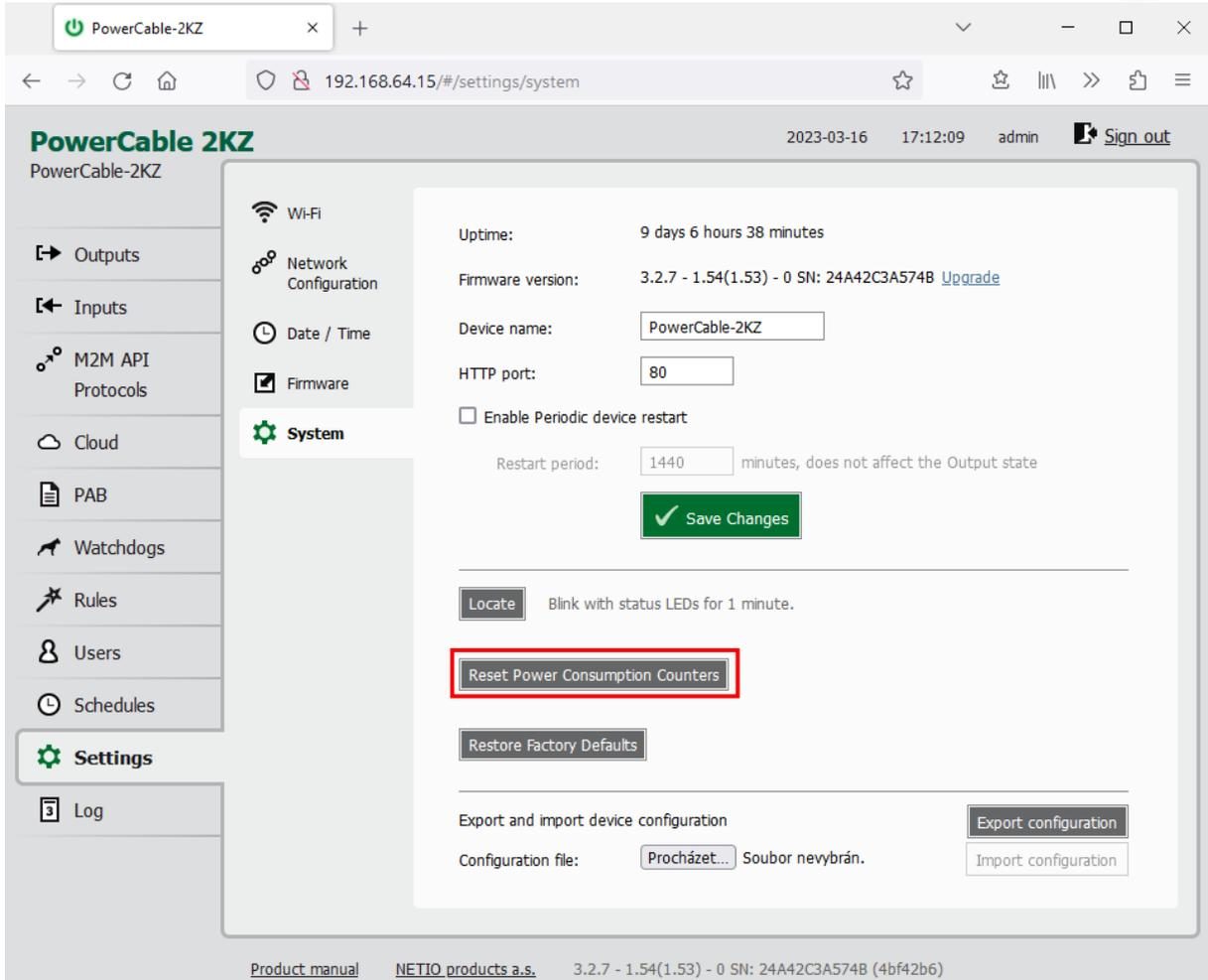
The screenshot displays the web interface for a PowerCable-2KZ device. The browser address bar shows the URL 192.168.64.15/#/settings/system. The page title is "PowerCable 2KZ" and the user is logged in as "admin". The left sidebar contains navigation options: Outputs, Inputs, M2M API Protocols, Cloud, PAB, Watchdogs, Rules, Users, Schedules, Settings (selected), and Log. The main content area shows the "System" configuration page with the following details:
