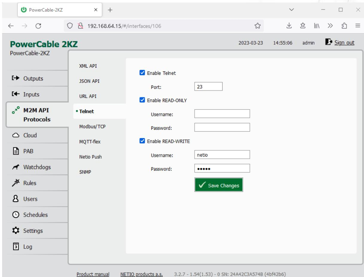
Figure 47 - Telnet protocol configuration
