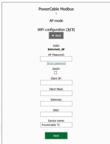
Figure 26 - Configuring the network IP parameters
