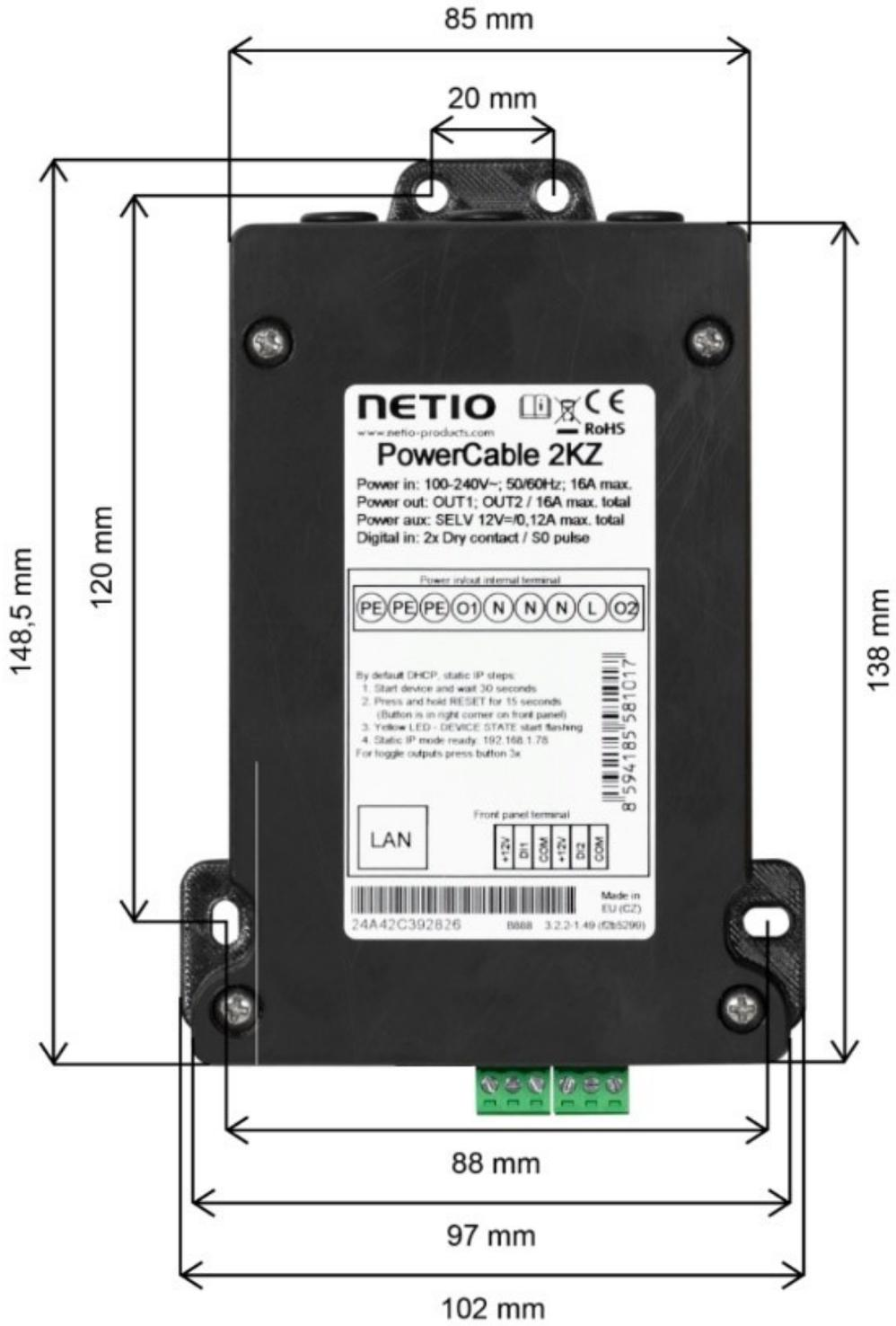
Figure 11 - PoweCable 2KZ top view
