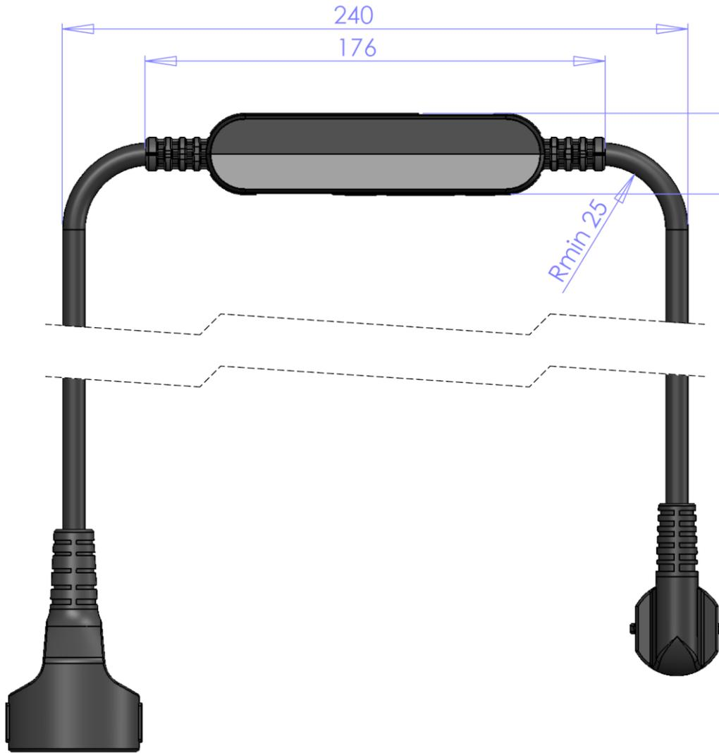
Figure 12 - PoweCable xxx 101x side view
