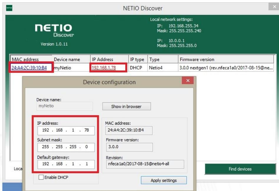
Figure 30 - Discovering network parameters using NETIO Discover
