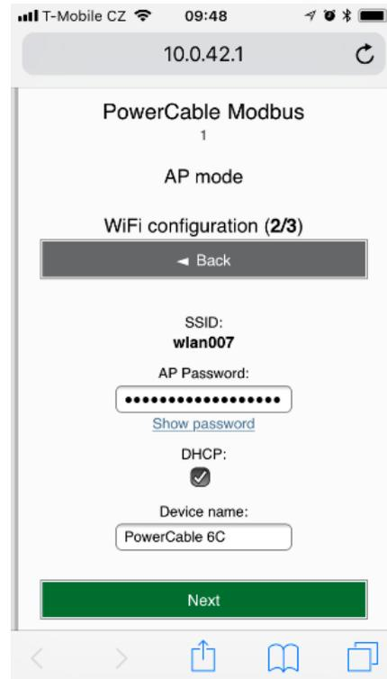
Figure 25 - Connecting to Wi-Fi in AP mode
