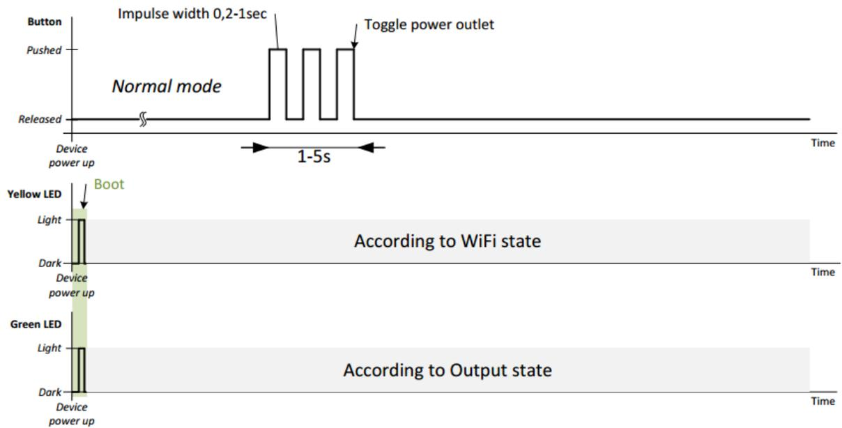
Figure 33 - LED indication for manual output control
