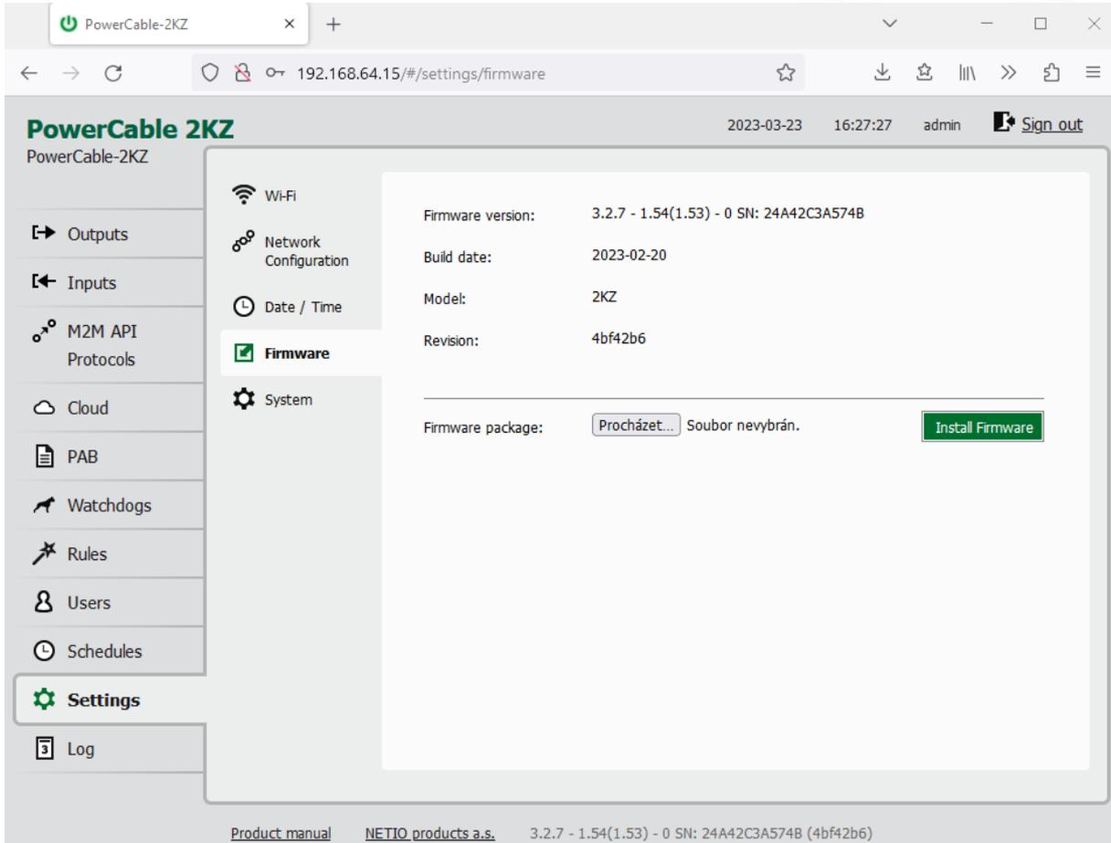
Figure 65 - Details about the installed firmware
